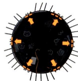
C) Continue connecting the leafsprings on the right sides of the joiners. Always connect the joiners that are on opposite sides to keep the tension on the mat even.
